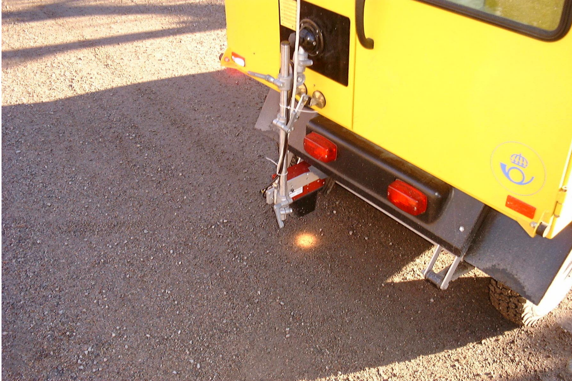
Figure 4: The speed measurement system mounted on the back of the Carryall vehicle
