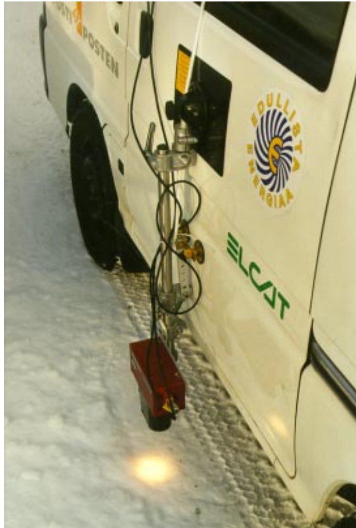
Figure 3: the speed sensor in use
