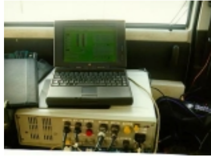
Fig. 13.7: On road DC-measuring system
