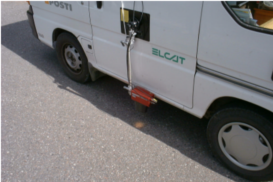
Figure 4: The speed measurement system
