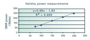
SMR power meter validation. SMR power was related to power delivered to the rear wheel by the velodyne, by the following equation :
