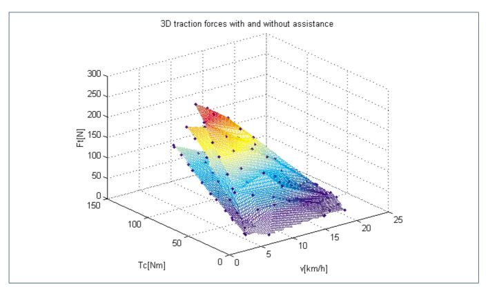
Output plot of EPAC (Yamaha PAS) in non-assisted, eco-assisted and assisted mode
