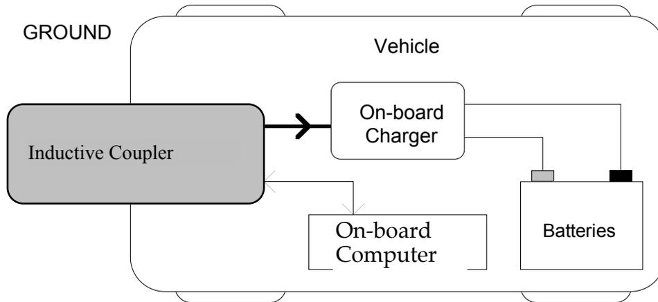
Figure 3 : Functional interface of recharging equipment with vehicle
