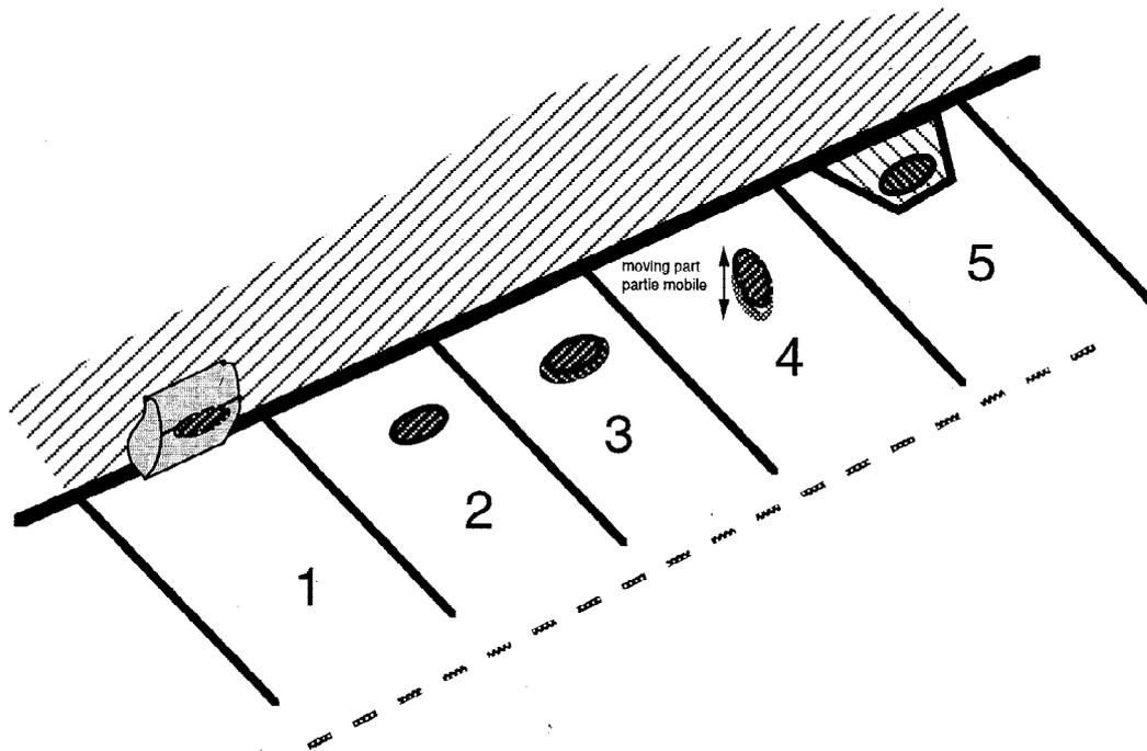
Figure 1 : Inductive charging configurations
