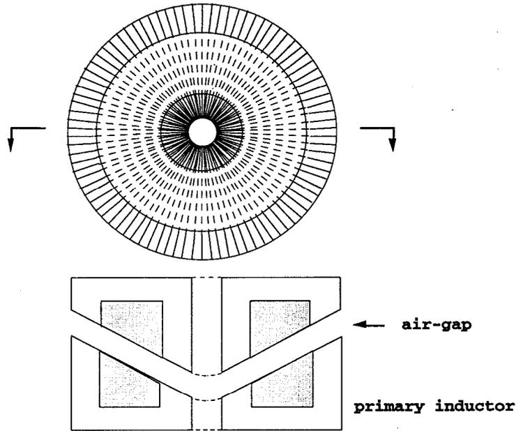
Figure 7 : Structure of the 400 Hz pot-core coupler
